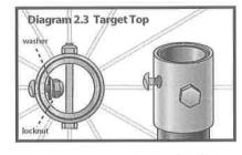
the target top , as you put the target top onto the pole. Line up the three holes on the target top with the top 3 holes on the pole. Insert and tighten  $1/4" \times 3/4"$  one-way screw into threaded hole on front of target top lining up with tab of locking collar. Start the 1/4" washer and locknut onto back of owe-way screw. (Do not tighten) Insert  $5/16" \times 2 \ 3/4"$  hex bolt through target top and pole tighten locknut. At this point tighten the 1/4" locknut onto one-way screw.
